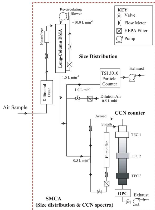
**Figure 1.** Schematic of the setup used for the Scanning Mobility CCN Analysis (SMCA).
