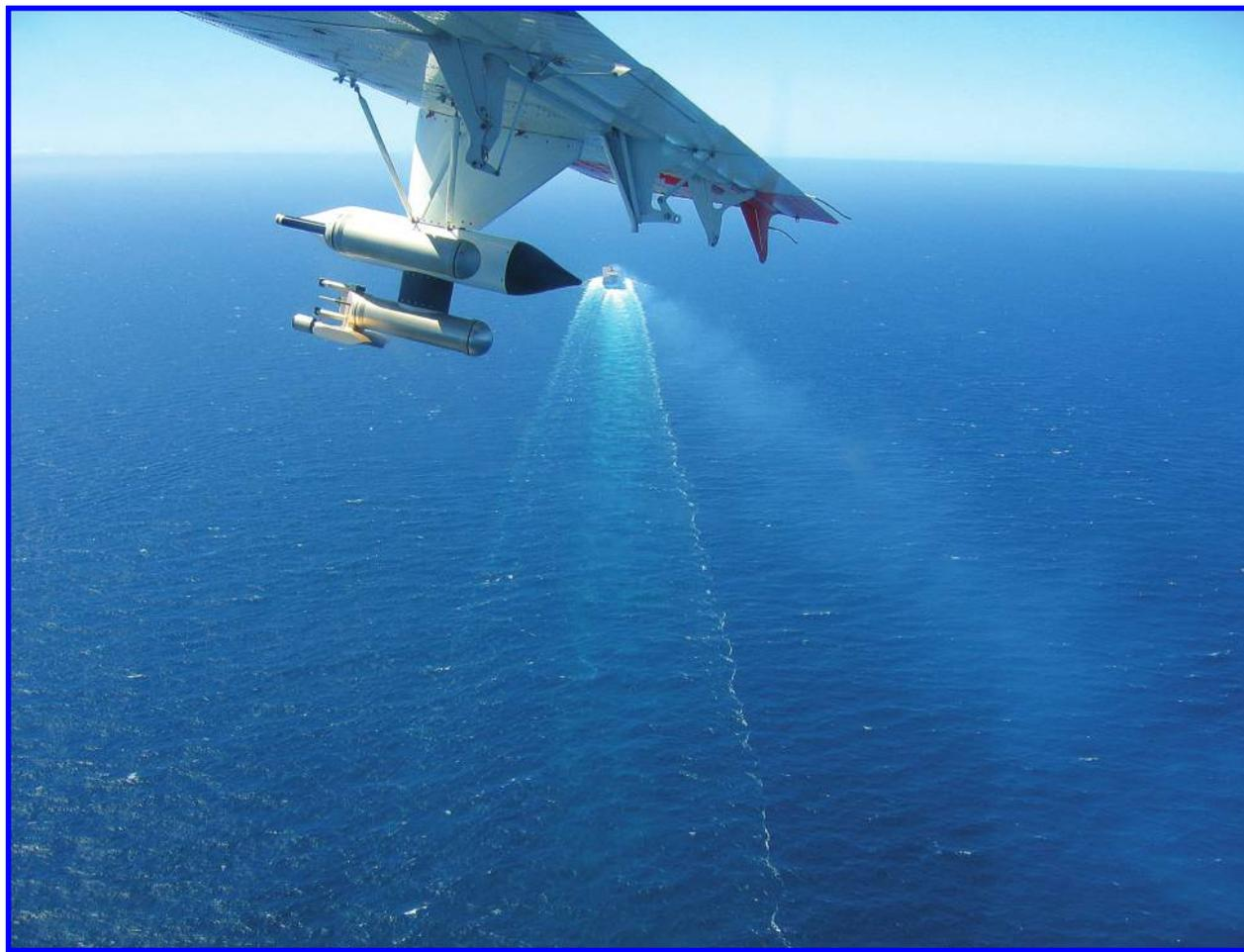
**FIGURE 1.** Photograph taken of the container ship from the cabin of the CIRPAS Twin Otter (the plane's wing tip is in the foreground) during the study. The exhaust plume is visible traveling with the mean wind at  $\sim 10^\circ$  angle to the heading of the ship, which can be inferred by the visible wake.
